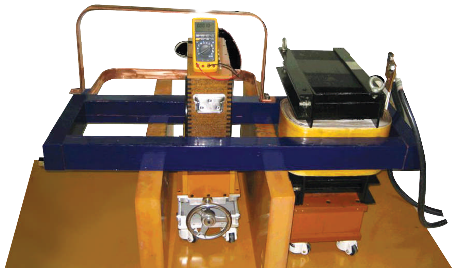
전압 전류발생장치 컨트롤판넬 / Voltage & Current Control Panel
